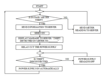
Above flowchart is used to detect power theft at pole as well as atconsumer meter in following way;
