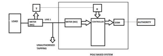
Fig (1). Block diagram of power theft detection.
